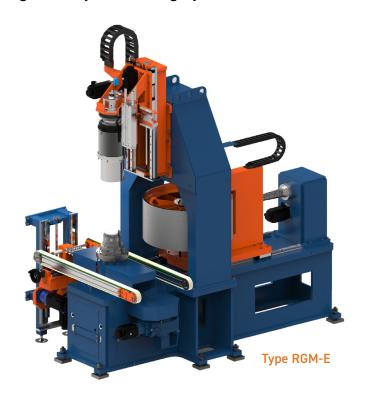
The Hofmann uniformity machine can easily be used with the Hofmann TU-TB interface and grading software and can be connected with a Hofmann balancing machine to an automatic tire grading line.
